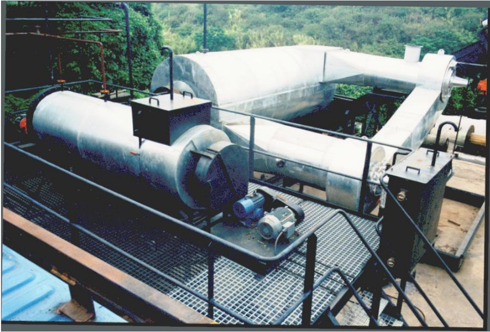
The FFS designed and built “PYROLISER”, showing the steam jacketed pin mill feeder (front left) and the hot air re-circulation system on the insulated rotary drum.
